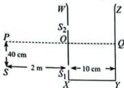
The distance between the slits is 0.8 cm. POQ is line perpendicular to the plane WX and passing through O, the middle point of  $S_1$  and  $S_2$ . A monochromatic light source is kept at S, S0 cm below S1 and S2 m from the vessel, to illuminate the slits as shown in the given figure.
